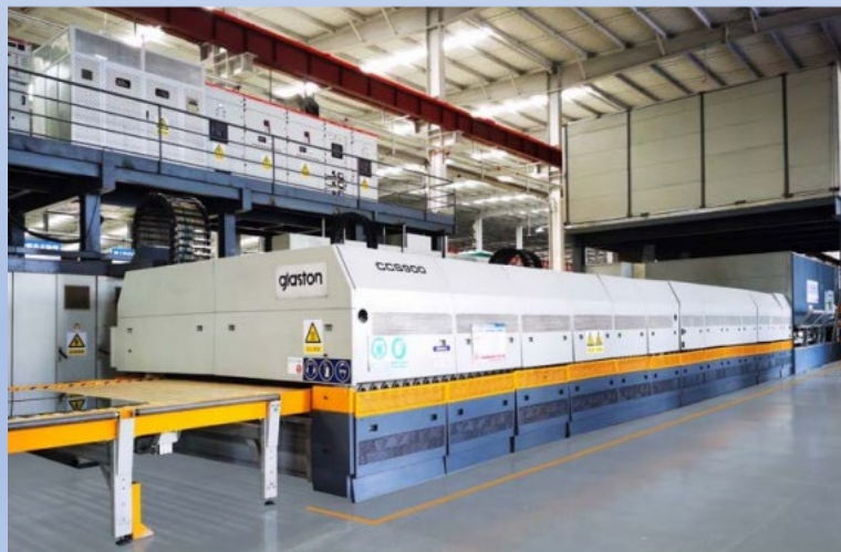
Glaston Tempered Furnace
